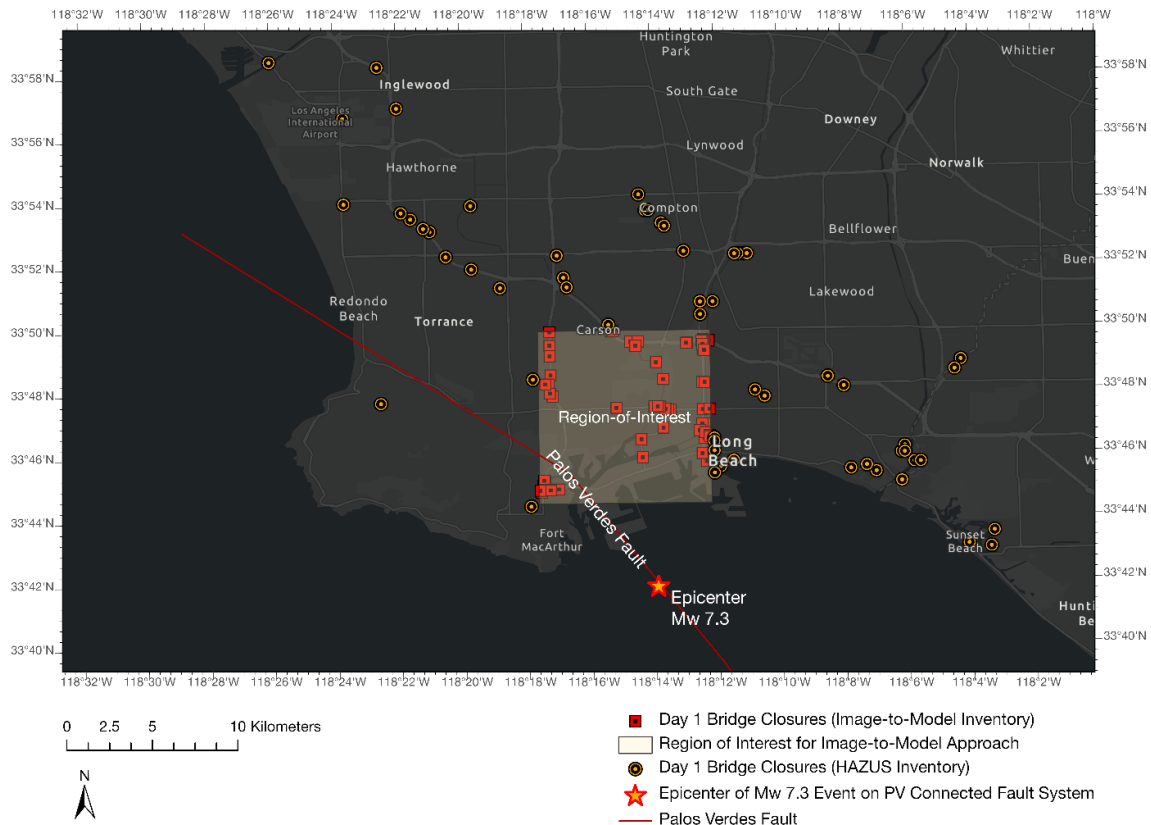
Figure 6. Modeled Bridge Closures on Day 1
